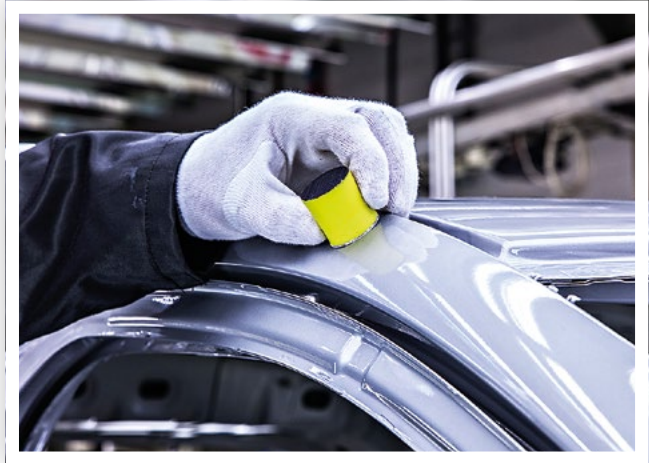
» Waterproof finessing discs enable a fast cut and a reliable finish. The product can be used wet or dry with an orbital sander or a random orbital sander.
