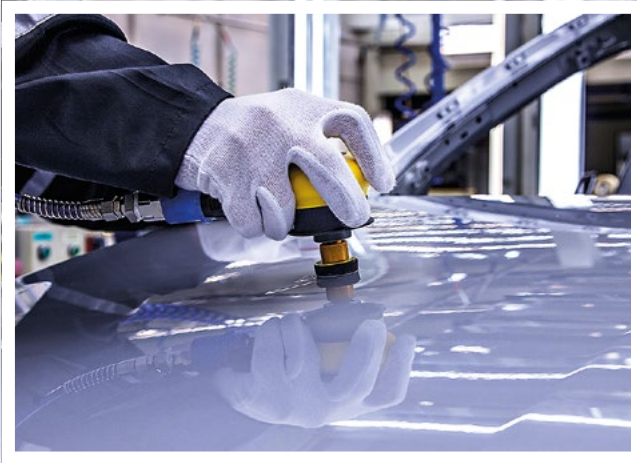
» Polarstar SR gives a high-quality finish enabling a fast polishing process. Mirka recommends the use of damp sanding with the orbital sander or random orbital sander.
