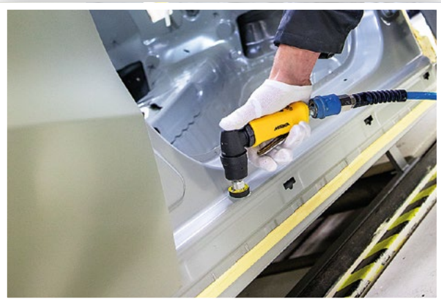
▶ Mirka® AOS 130NV with Polarstar P400. Sanding in hard-to-reach areas.
