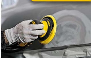
Paint removal / Feather edge
